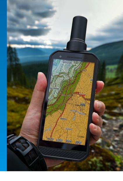
The RDC 50 GIS handheld device is equipped with a high-performance positioning chip, supporting five major GNSS satellite systems and dual-frequency L1+L5 positioning. With instant fix technology, precise operations require no waiting. The device also features 4GB RAM and 64GB of large storage, enabling seamless execution of raster and vector data tasks in a single device.
